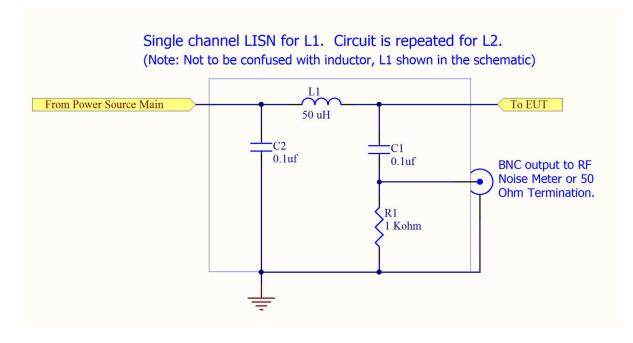
Figure 1. Circuit model of an LISN as outlined in ANSI C63.4-2003.
