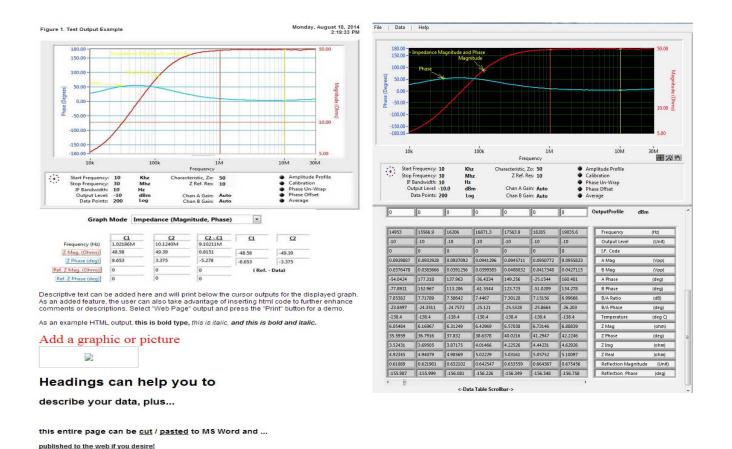
Figure 5. Webpage output showing graph output, HTML enhancement capability, and screen with scrollable tabular data. Data is also exportable to csv file for spreadsheet apps.
