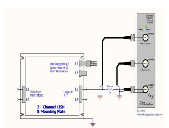
Figure 2. Test setup for measuring the EUT terminal impedance.
