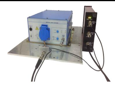
Conducted emissions is a measure of the amount of Electromagnetic Interference (EMI) that is conducted from a unit under test (EUT) to the outside world via the power cables. A Line Impedance Stabilization Network (LISN) is used for conducted emissions testing, and is inserted between the power mains and the EUT.
