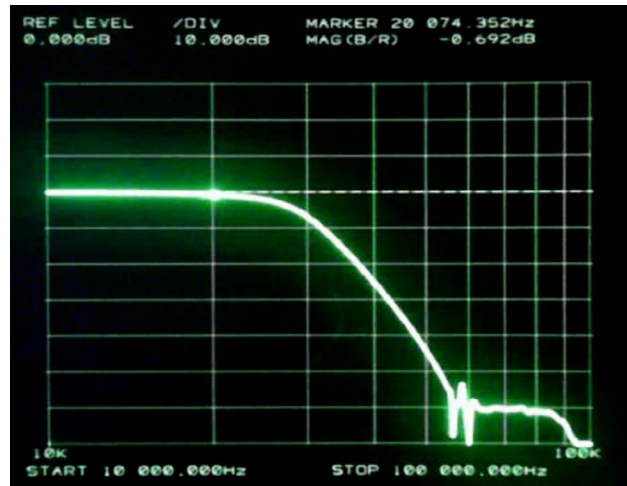
Figure 4. Frequency response from 10kHz to 100kHz showing gain flatness to 20kHz. +4dBm (1Vpp) input signal.
